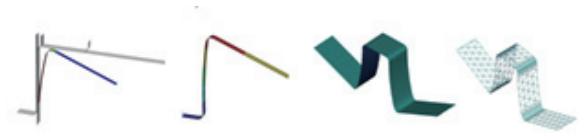
Fig. 2 U-bending benchmarking problem using (a) ABAQUS and (b) AutoForm
