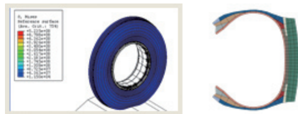
Fig. 1-2 FE Tire Model
