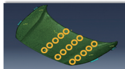
Fig. 5 simulation for obtaining stiffness of hood.
