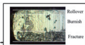
Fig. 6 Spacer grid (left) and sheared edge formation after blanking process (right)
