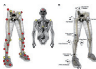
Fig 20 Human lower-extremity model using marker based motion capture system
