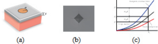
Fig. 3 Application of nano-indentation (a) Film-on-substrate system (b) Indentation crack and (c) Residual stress
